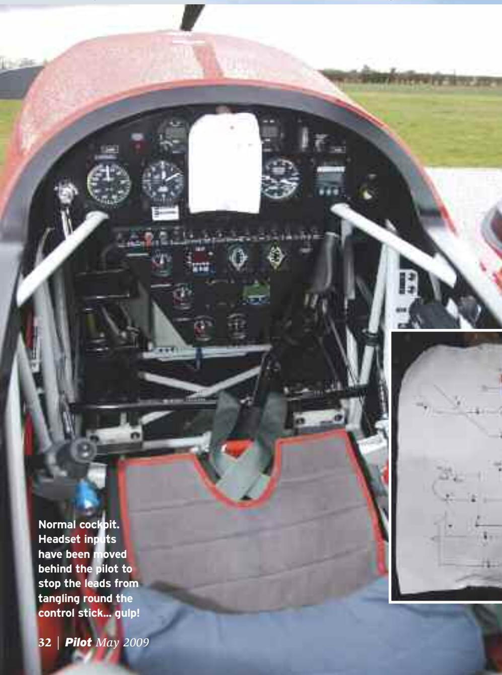
Normal cockpit. Headset inputs have been moved behind the pilot to stop the leads from tangling round the control stick... gulp!
