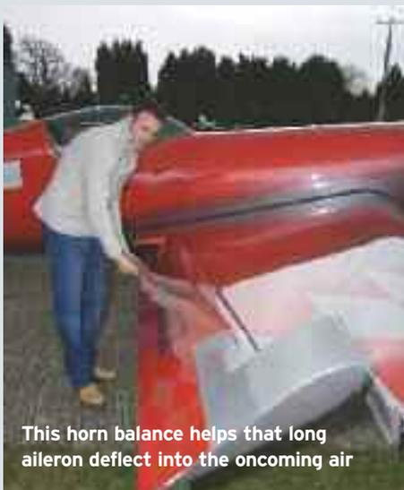
This horn balance helps that long aileron deflect into the oncoming air
