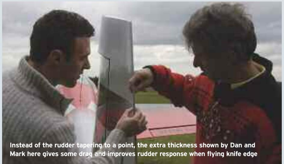
Instead of the rudder tapering to a point, the extra thickness shown by Dan and Mark here gives some drag and improves rudder response when flying knife edge
